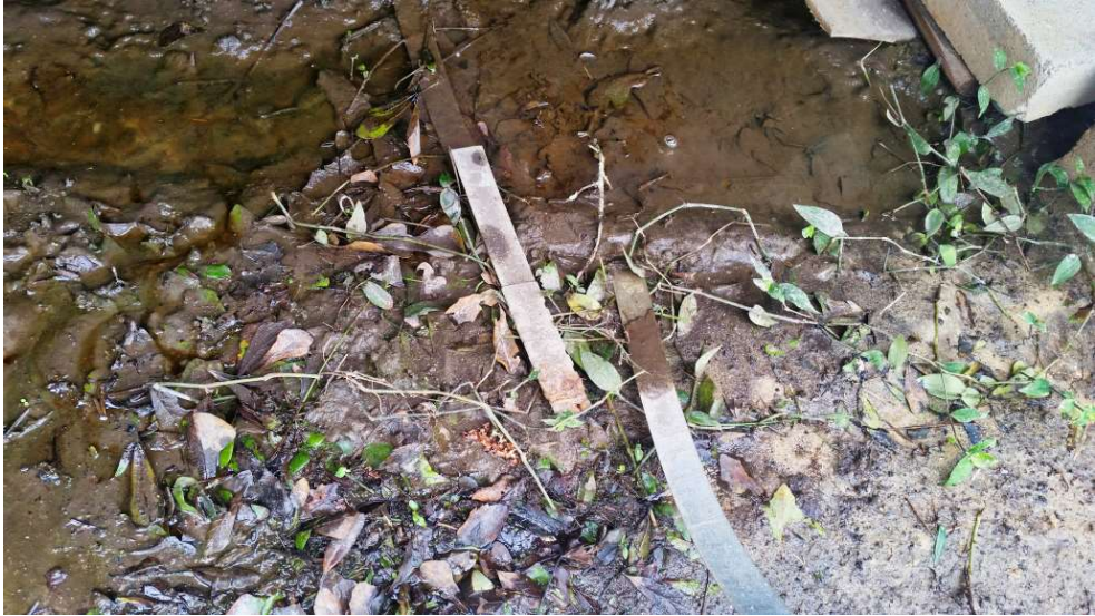
Strap Parted due to Rust
